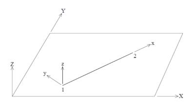
Figure 9: Local axes of elements in 2D models
