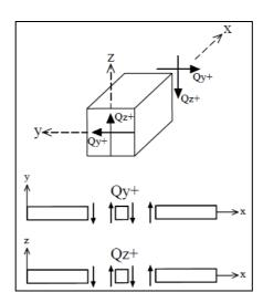
Figure 15: Positive internal shear force
