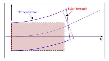
Figure 8: Comparison between Euler-Bernoulli element and Timoshenko element
