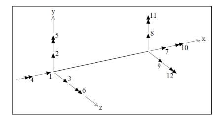
Figure 6: Degrees of freedom positive directions of a 3D frame element in local system
