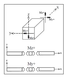
Figure 16: Positive internal bending moment
