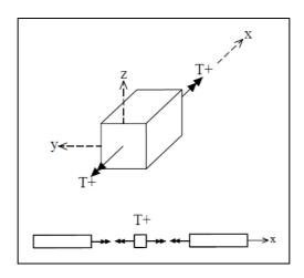
Figure 14: Positive internal torsion moment
