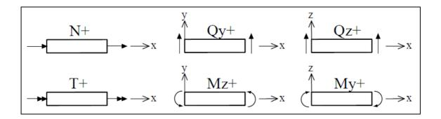
Figure 18: Positive internal forces convention in textual results
