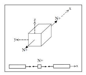
Figure 13: Positive internal axial force
