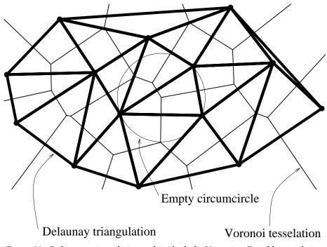
Figure 23: Delaunay triangulation and its dual, the Voronoi or Dirichlet tesselation.
