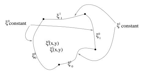
Figure 7: Elliptic grid generation boundaries
