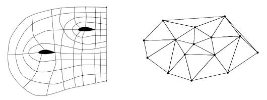
Figure 1: Structured mesh (left) and unstructured mesh (right).
