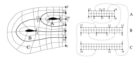
Figure 15: Example of multiblock: 3 C-type grids
