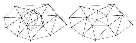
*Figure 27: Bowyer-Watson triangulation: circumcircles that contain the new point, and the resulting triangulation*
