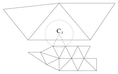
*Figure 22: Element generation failure (side intersection) because of too small a value of search radius.*
