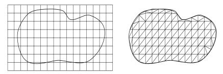
Figure 17: Overlaid grid, cropped, warped to boundary and split into triangles
