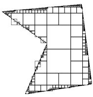
Figure 18: Quadtree grid, before triangulation and warping
