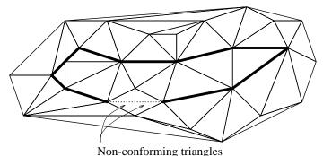
Figure 28: Delaunay triangulation not conforming to a boundary
