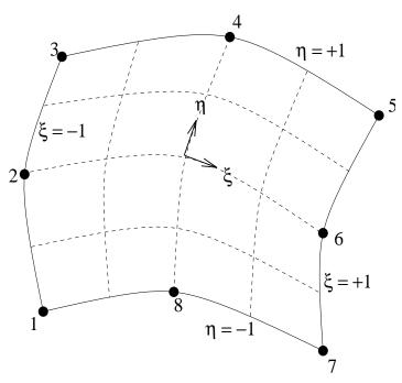
Figure 16: Isoparametric meshing
