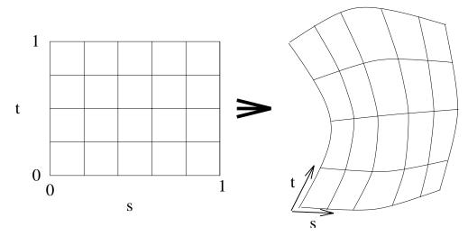
Figure 5: Transfinite interpolation
