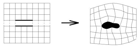
Figure 2: Two-block boundary-fitted grid
