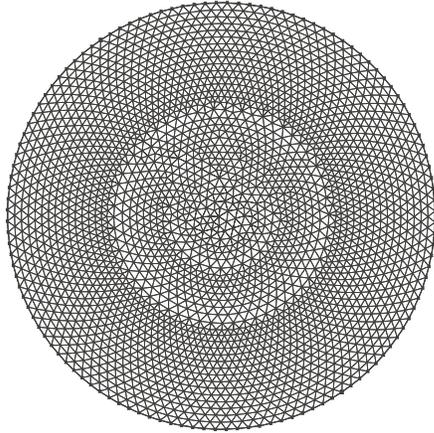
Figure 14: Mesh for the circle model.
