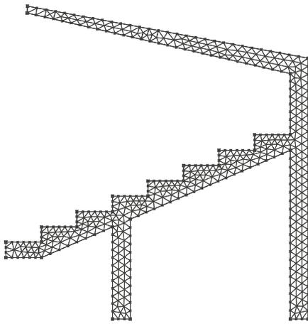
Figure 15: Mesh for the stand model.
