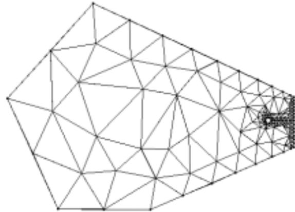
Figure 8: First mesh generated for the example.
