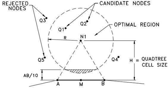
Figure 5: The determination of a triangle.
