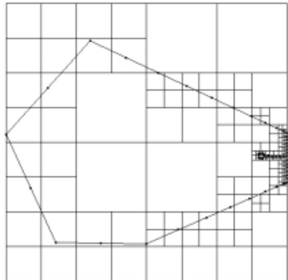
Figure 2: Initial quadtree of model.
