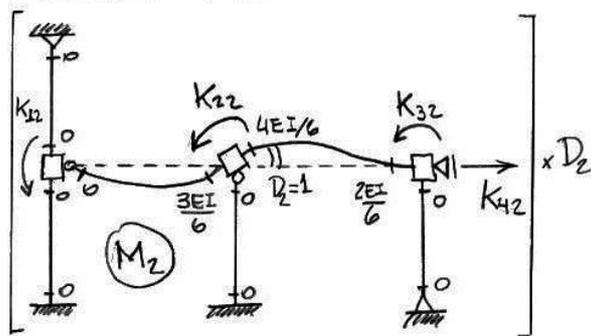
$$\begin{aligned} K_{12} &= 0 \quad K_{22} = \frac{3EI}{6} + \frac{4EI}{6} = \frac{7EI}{6} \\ K_{32} &= \frac{2EI}{6} \quad K_{42} = 0 \end{aligned}$$
