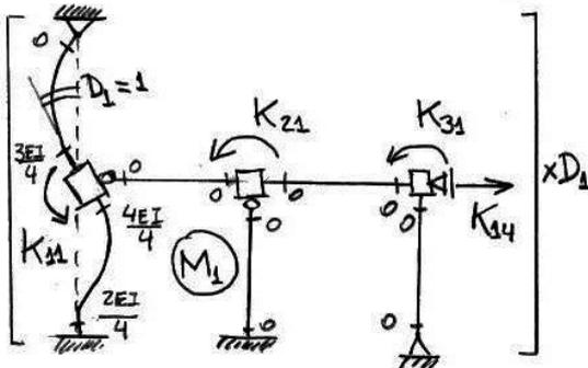
$$\begin{aligned} K_{11} &= \frac{4EI}{4} + \frac{3EI}{4} = \frac{7EI}{4} \\ K_{21} &= 0 \quad K_{31} = 0 \\ K_{41} &= \frac{6EI}{4^2} - \frac{3EI}{3^2} = \frac{3EI}{4^2} = \frac{3EI}{16} \end{aligned}$$
