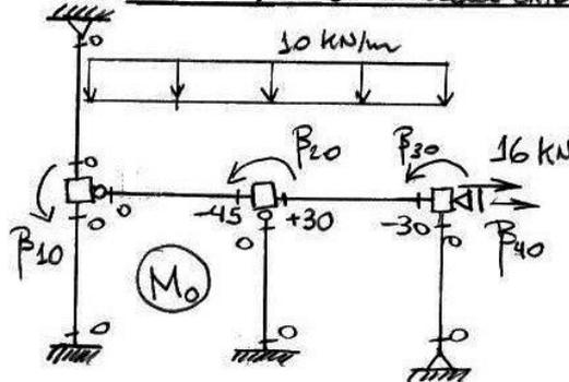
$$\begin{aligned} P_{10} &= 0 \\ P_{20} &= -45 + 30 = -15 \text{ kNm} \\ P_{30} &= -30 \text{ kNm} \\ P_{40} &= -16 \text{ kN} \end{aligned}$$
