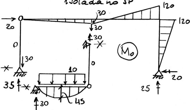
$$EI\delta_{10} = -\frac{1}{2} \times 6 \times 120 \times 1 + \frac{1}{2} \times 6 \times 30 \times 1 - \frac{1}{3} \times 6 \times 120 \times 1 = -510$$
