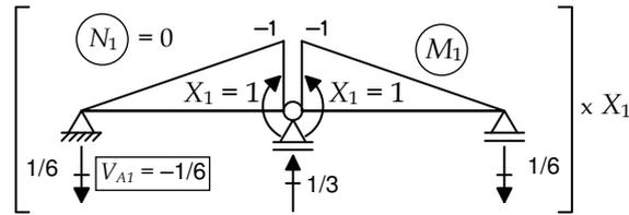
$$\delta_{11} = \int_{\text{viga}} \frac{(M_1)^2}{EI} dx + \int_{\text{viga}} \frac{(N_1)^2}{EA} dx$$
