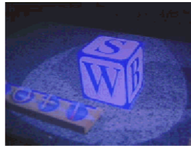
Image seen by a head tracked user standing to the right of a cube located on the surface of the bench display.
