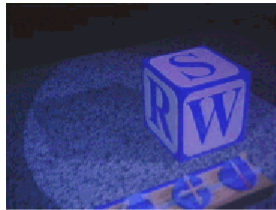
Image seen by a head tracked user standing to the left of a cube located on the surface of the bench display.
