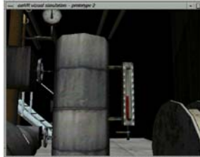
Fig. 8 : The user has to control liquid in the check glass, which is mounted on the container.
