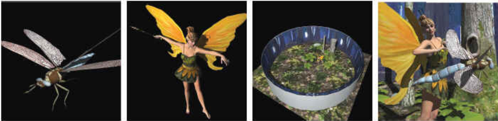
Fig. 7. Fairy-forest test scene. An animated dragonfly (a) and a dancing fairy (b) placed into a typical game environment with background textures and animated foreground geometry (c). The resulting scene (d) consists of 180,000 animated triangles and is rendered with textures, shading, and shadows, at 2.2 fps at 1024 \times 1024 resolution.
