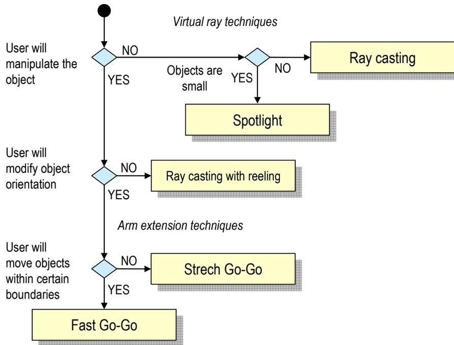
**Figure 6.2** Design guidance tool for object selection and manipulation techniques
