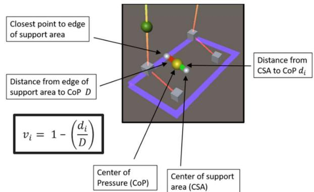
Fig. 3 Calculation of balance state
