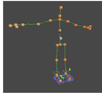
Fig. 5 Joints tracked by the MS Kinect SDK.
