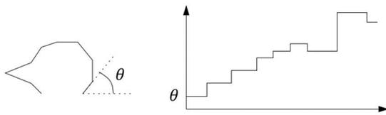
Fig. 16 Curve and turning function
