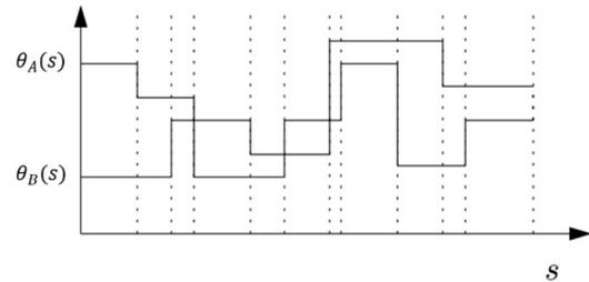
Fig. 17 Evaluation of dissimilarity with turning functions
