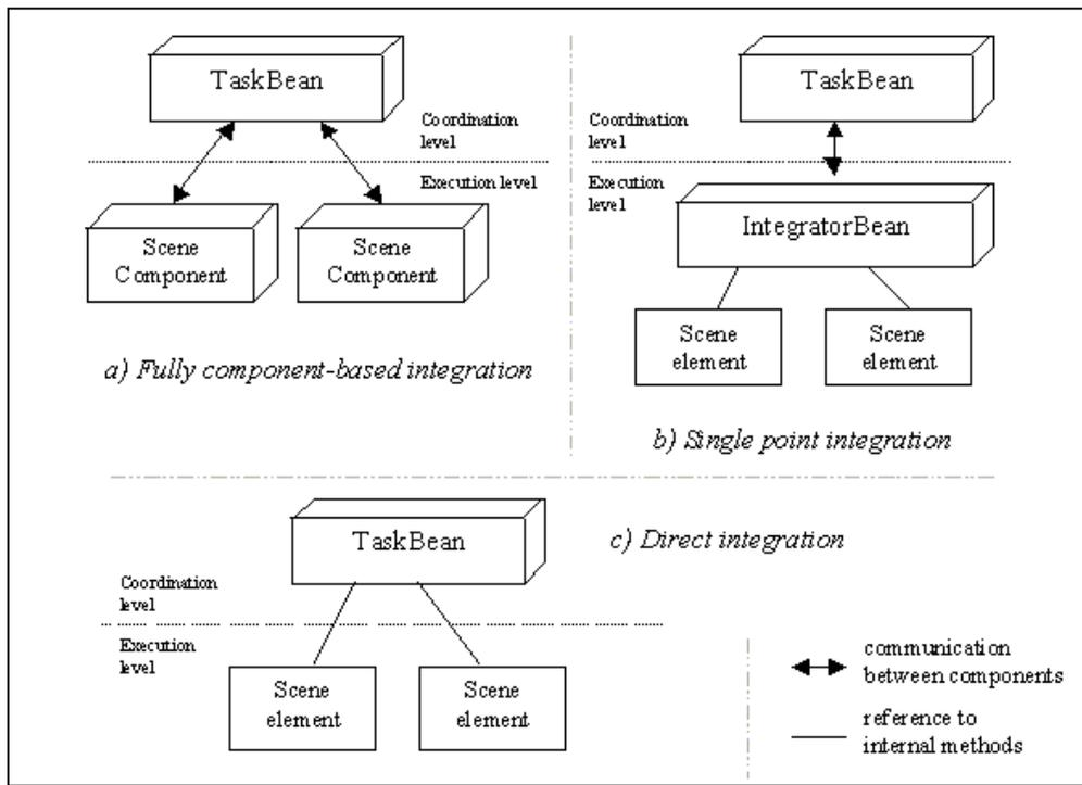
**Figure 3:** Approaches for the integration of scene-coordination components.
